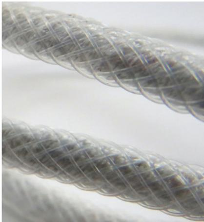
The unique, robust construction of the **Floodline One-Zone Absorbent Leak Detection Cable** has 2 cores twisted around a central former, wrapped in an absorbent outer braid.
