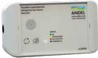
The Floodline RGD1601 gas detector can be used as either a stand-alone gas sensor or connected to Floodline alarm panel and can be powered by 110-230Vac or 12-24Vdc. The Floodline RGD1601 is intended for VRV air conditioning systems and refrigeration compressor packs. The unit can be calibrated to detect one of either R134a, R410A, R407c or R404a gases.
